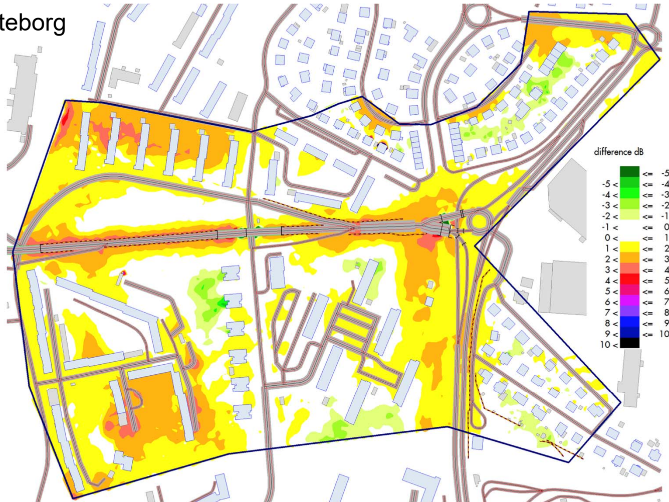
Figure 7: Differences between two noise contour calculations – a calculation made with RTN96, minus a calculation with CNOSSOS-EU using default values of p_f . Arithmetic mean of all calculated points is 1,1 dB, median 1,1 dB, and standard deviation 1,5 dB. Noise protection walls are shown as black-yellow dashed lines.
